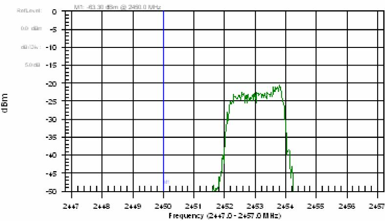
CF: 2452.0 MHz SPAN: 10.00 MHz Attenuation: 31 dB RBW: 10 kHz VBW: 3 kHz Detection: Pos. Peak
