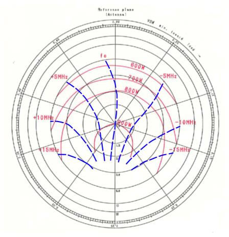
Change in load reactance, changes the frequency. Change in frequency depends upon amount of power reflected and its phase.
